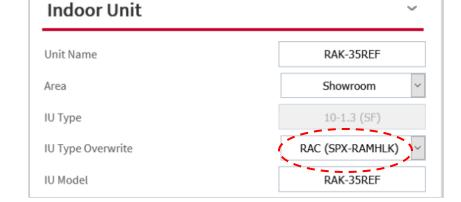
Silent fan speed and louver control are not available from CSNET Manager and CSNET Lite for RAC units (with SPX-RAMHLK and PSC-6RAD):
