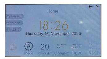
Auto Cool/Heat operation mode can be applied to the Yutaki space heating zone, from LCD controller or from the App
