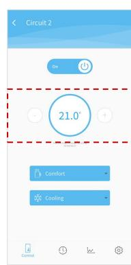
Zone 1 with RTU, heating OTC=gradient, cooling OTC=fixed water temp. Fixed water set point is only displayed for cooling mode (Settings page)
